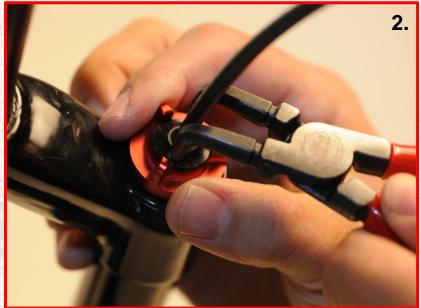
Remove the cable completely from the fork.
